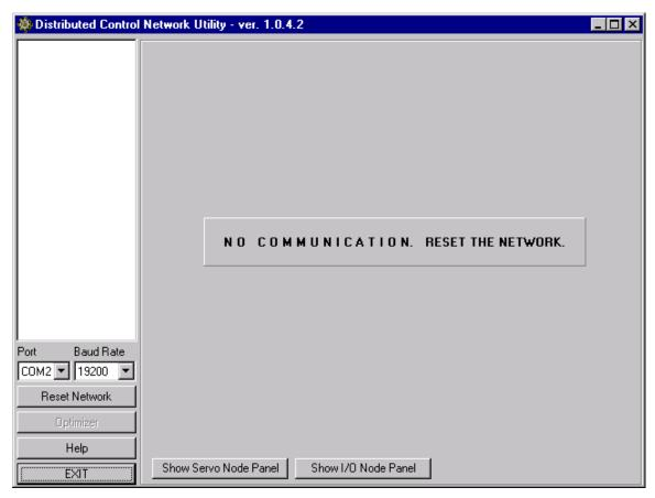
Then you need to check your Com Port settings and your baud rate (lower left of screen), check your cabling to make sure you have a good connection between your Com Port on the PC and the DB-9 Connector on the Servo Box. Once this all has been verified, choose the Reset Network button.
