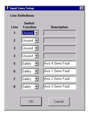
Please note that if you are using the FlashCut CNC Limit Switch Kit with 5 switches and you have a 4 Axis controller, the Z+ limit switch and the Axis 4 Servo Fault would share the same line. In this case it is best to disconnect the Axis 4 Servo Fault by
